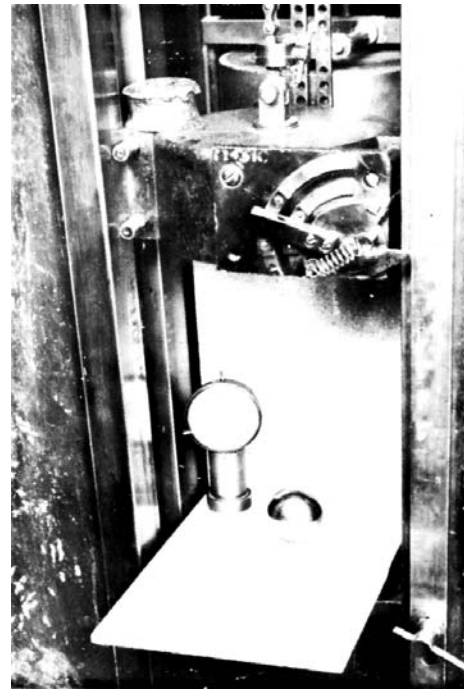
FIG. 5 Apparatus for Falling-Ball Indentation Test for Wood or Wood-Based Finish Flooring
