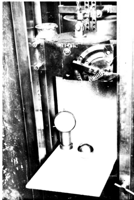
FIG. 5 Apparatus for Falling-Ball Indentation Test for Wood or Wood-Base Wood-Based Finish Flooring
