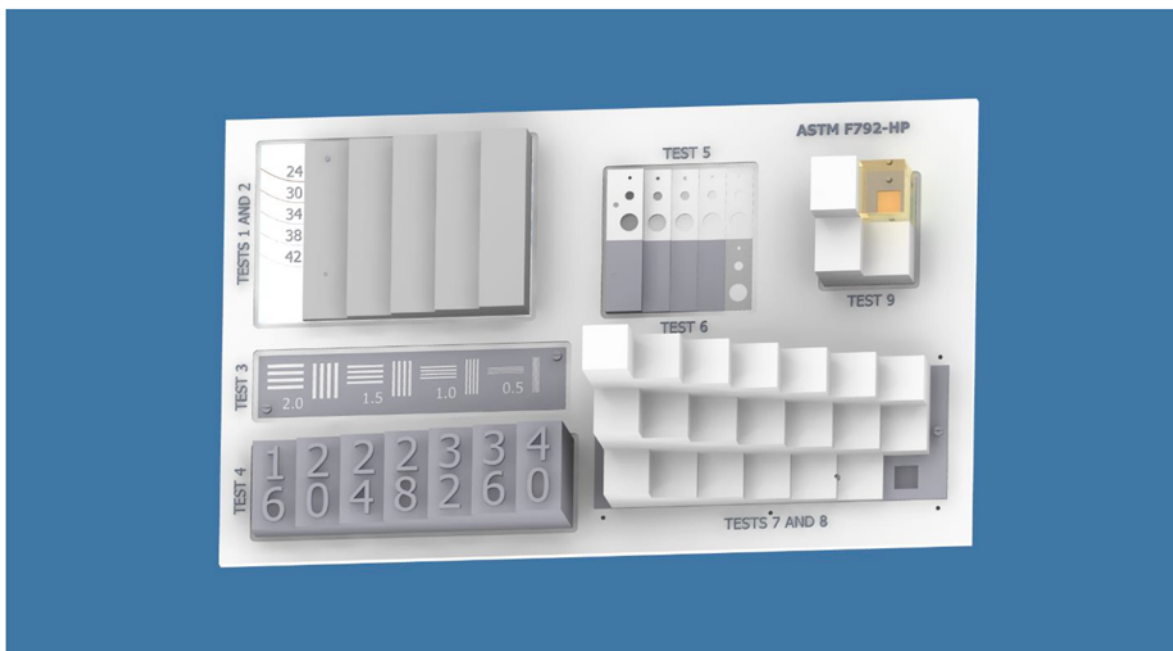
The test pieces for all nine tests are labelled on the test object and are described in more detail in subsequent sections.
