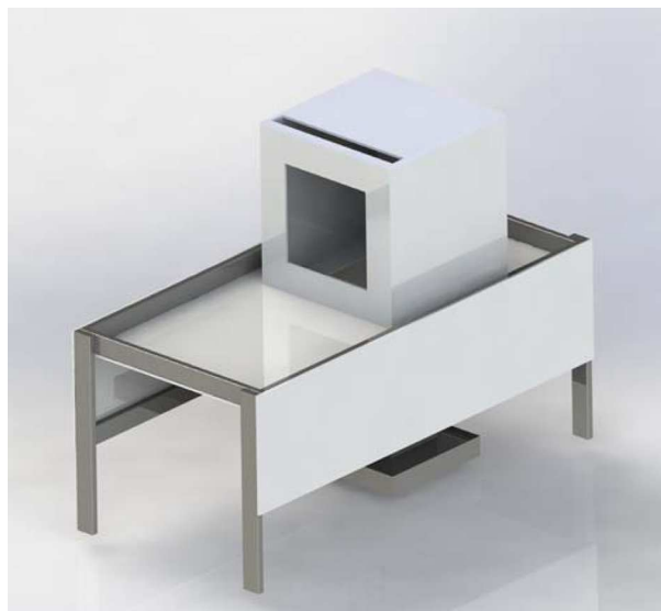
FIG. 9 Example of Test Bench, Fire Source, and Test Box in Test Configuration
