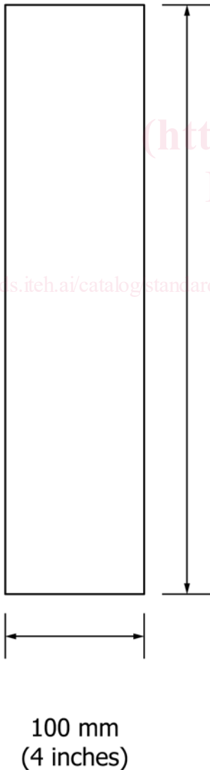
FIG. 2 Cut Specimen Dimension from Fabric
