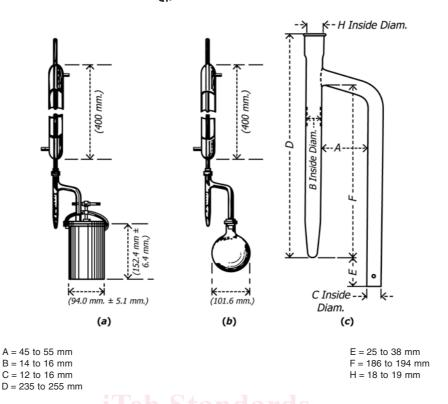
FIG. 1 Apparatus for Determining Water Content
