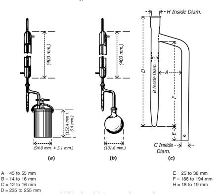
FIG. 1 Apparatus for Determining Water Content
