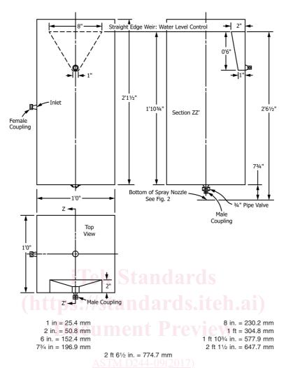
Note 1—Use galvanized steel sheeting for the tank. All joints and fitting attachments shall be soldered and shall be watertight. All couplings shall be standard brass garden hose fittings. The 19-mm pipe valve shall be placed as close as possible to the bottom of the tank, allowing space to shut off the valve. The tank shall be placed on a suitable stand, so that the distance from the bottom of the spray head to the top of the test sample is  $0.914 \text{ m} \pm 25.4 \text{ mm}$ .
