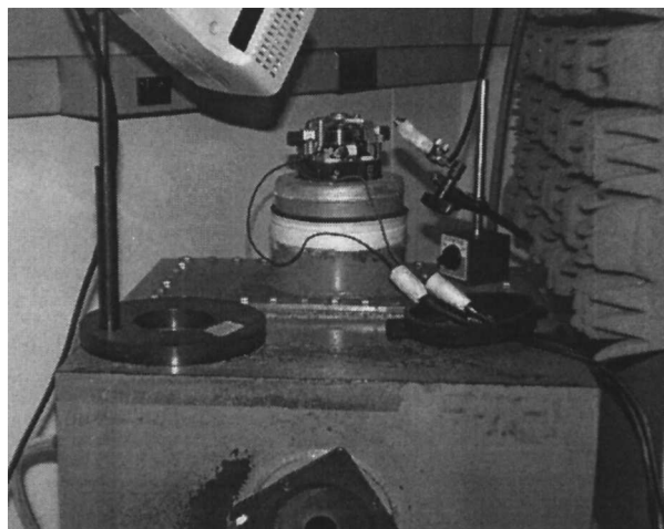
FIG. 1 Motor Mounted to Plenum Chamber
