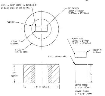
Note 1—The dimensions for the cavity shall be  $0.500 \pm 0.004$  in. wide  $(12.70 \pm 0.10 \text{ mm})$  by  $1.250 \pm 0.004$  in. long  $(31.75 \pm 0.10 \text{ mm})$ . The mating parts shall fit freely and should be finished to a 4 uin. (N3) or better to dimensions of 0.0005 in. (0.013 mm) to 0.0010 in. (0.025 mm) smaller than the die cavity in each dimension. The dimensions given in the drawing typify the die cavity and punch within the stated tolerance at the normal width and length.
