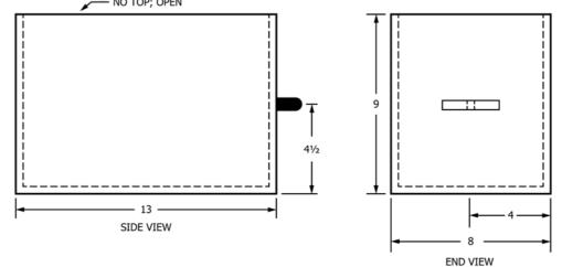
NOTE 1—Material specified is type 316 stainless steel (S.S.) or other suitable alloy (¼ in. (6 mm) recommended). Note 2—All dimensions minimum outside diameter.
