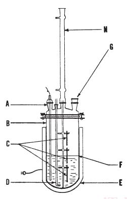
Note 1—The flask can be used as a versatile and convenient apparatus to conduct simple immersion tests. Configuration of top to flask is such that more sophisticated apparatus can be added as required by the specific test being conducted. A = thermowell, B = resin flask, C = specimens hung on supporting device, D = air inlet, E = heating mantle, F = liquid interface, G = opening in flask for additional apparatus that may be required, and H = reflux condenser.
