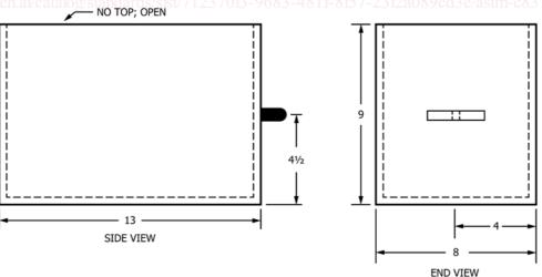
Note 1—Material specified is type 316 stainless steel (S.S.) or other suitable alloy (¼ in. (6 mm) recommended).
