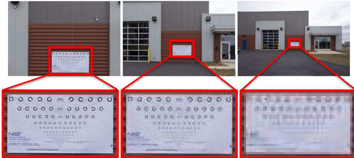
FIG. 43 Geometry of Three Images of the Same Scene with the Same Image Resolution. Top Row Shows Field of View Determination Increasing from Left to Right (the image “zooms out”) While Bottom Row Shows Acuity Decreasing (features of the same size become harder to clearly observe)
