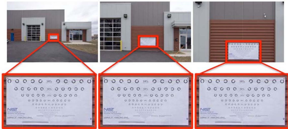
FIG. 4 Three Images of the Same Scene with the Same Field of View. The Top Row Shows the Field of View is Unchanged While Bottom Row Shows Both Resolution and Acuity Increasing (features become clearer)
