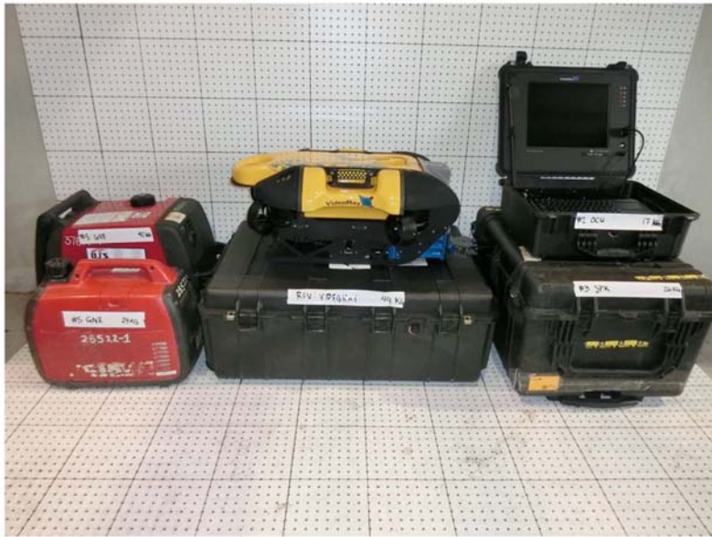
NOTE 1—All items in the system as they arrived on site for testing. They are staged in the photo booth with metered backdrop (20 cm [8 in.]). The chassis for the Remotely Operated Vehicle (ROV) under test is sitting on top of its packaging to show the correspondence. Each of the packages is clearly marked with a respective identification number, name, weight, type, and model.
