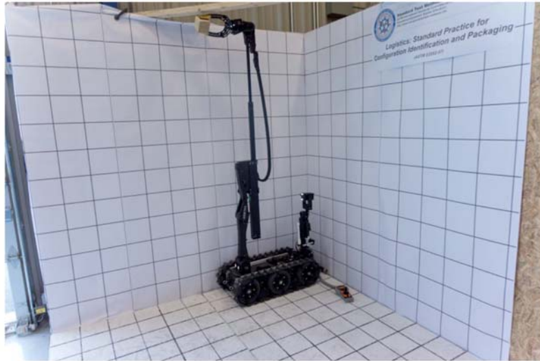
FIG. 1 Example of a Standard Environment in which a Robot May be Photographed for Documentation
