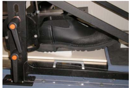
FIG. 1 Example of Footwear Mounted Using 7° Wedge to Set Proper Contact Angle
