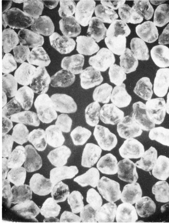
FIG. 6 25X Magnification AFS 50/70 Test Sand Ottawa Silica Co.
