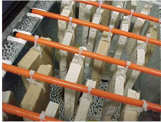
FIG. 3 Cable Ties used to Hang Test Specimens from Rods Inside of the Environmental Chamber
