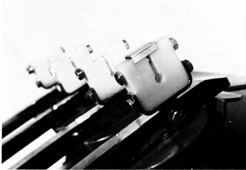
FIG. 5 Wear Block/Wear Specimen Holder
