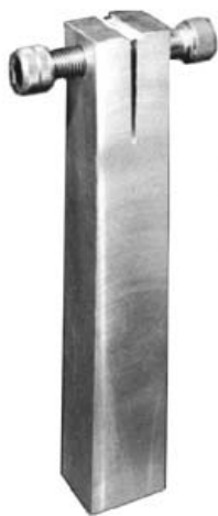
FIG. 4 Bolt Loaded Precracked Double Beam Specimen
