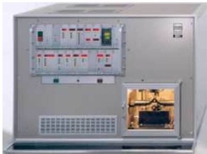
FIG. 1 SRV Model III Test Machine
