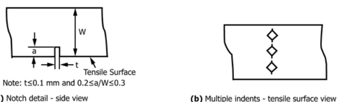
FIG. A2.3 Precracked Beam Precracking Arrangement
