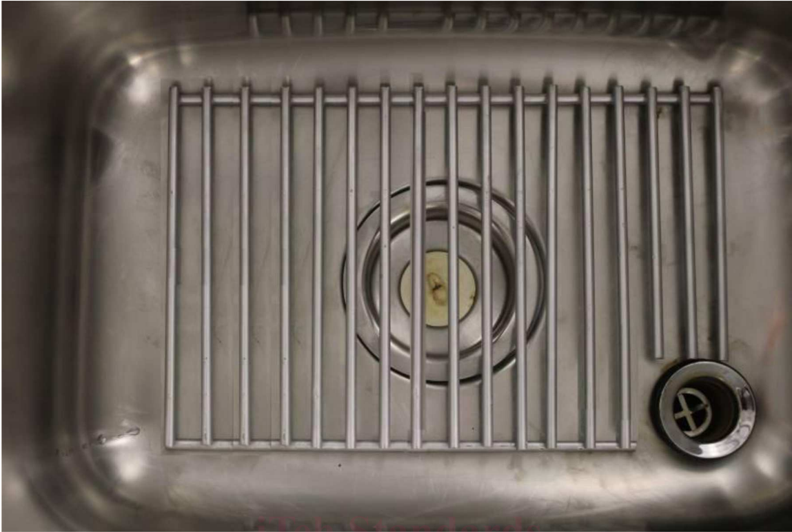
FIG. 4 Freezing Container with Tile Support Rack Installed
