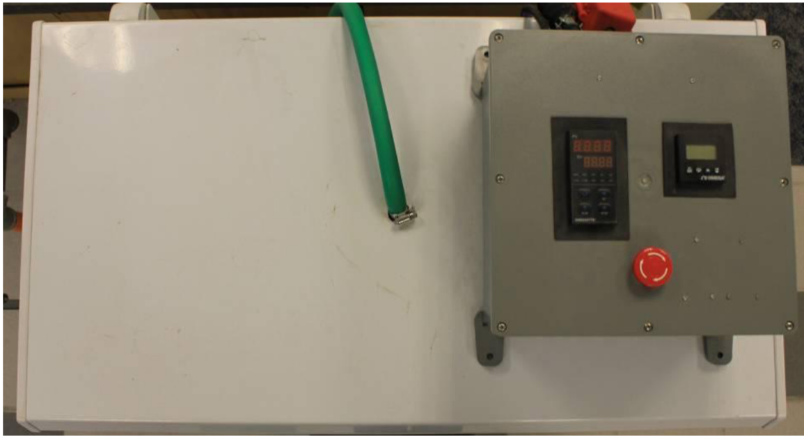
FIG. 2 Freezing Chamber, Top View Includes Inlet Hose from Water Pump and Control Box Housing the Temperature Controller and Cycle Counter
