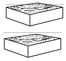
hole—a deep depression or void, the bottom of which is not visible by normal (20/20) vision under 200 fc illumination.
