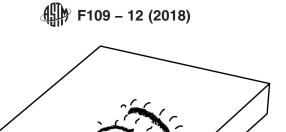
**crazing**—the cracking that occurs in fired glazes or other ceramic coatings as a result of tensile stresses, may also occur in the surface portion of uncoated (unglazed) whiteware bodies.
