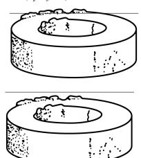
**flow line**—one or more streaks distinguished by a difference in light reflectance from the surrounding area, charateristic of injection-molded parts. (See also **weld mark**.)
