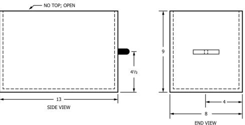
Note 1—Material specified is type 316 stainless steel (S.S.) or other suitable alloy ( $\frac{1}{4}$  in. (6 mm) recommended). Note 2—All dimensions minimum outside diameter.
