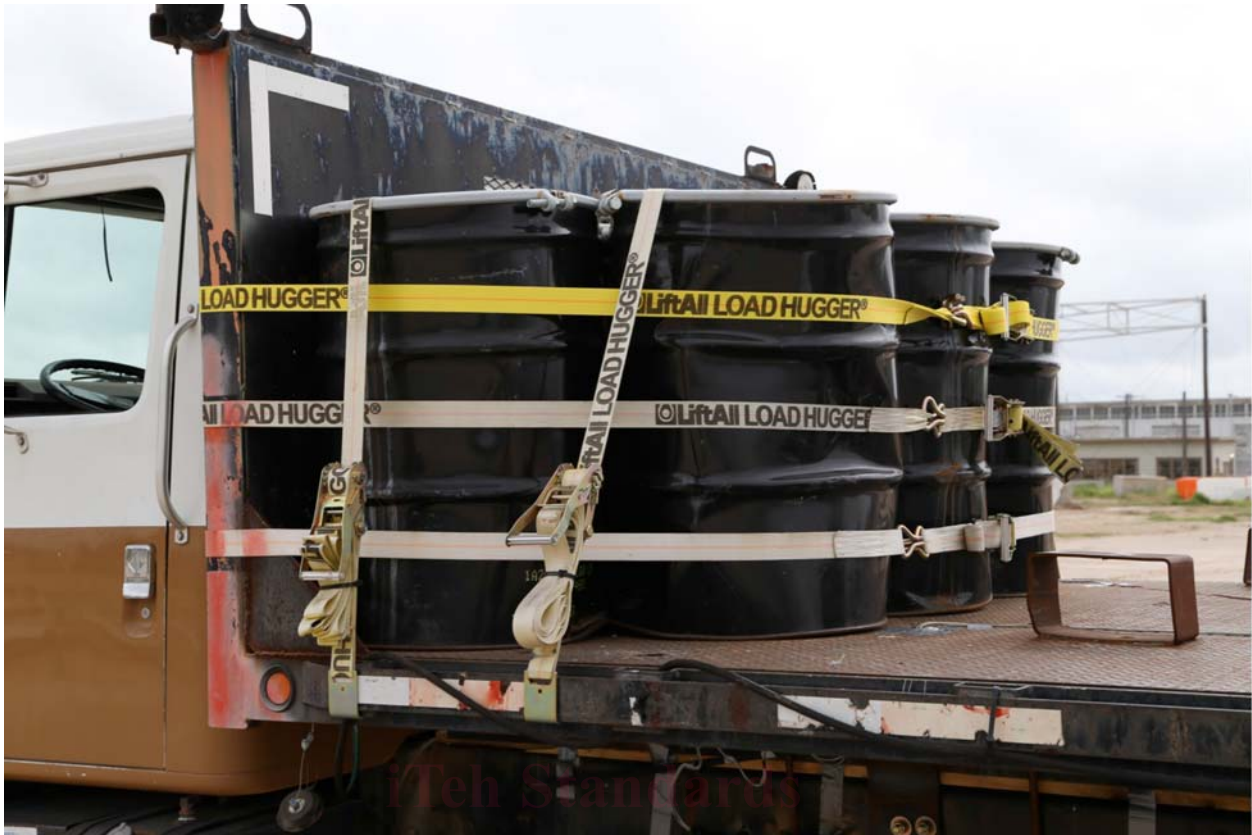
FIG. 2 Typical Ballast Attachment, Rear View
