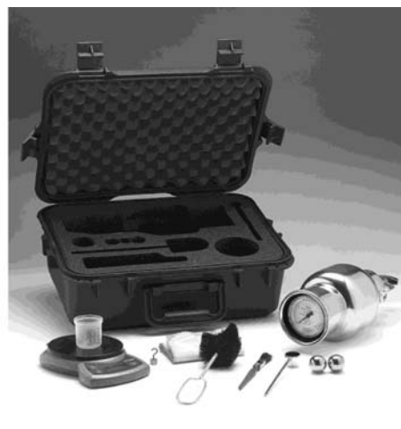
FIG. 1 Typical Calcium Carbide Gas Pressure Test Apparatus for Water Content of Soil
