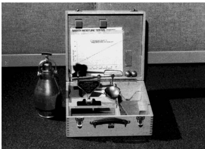
FIG. 1 Typical Calcium Carbide Gas Pressure Test Apparatus for Water Content of Soil
