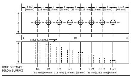
Note 1-Entrant surface shall be 250 µin. [6.3 µm] or finer.
