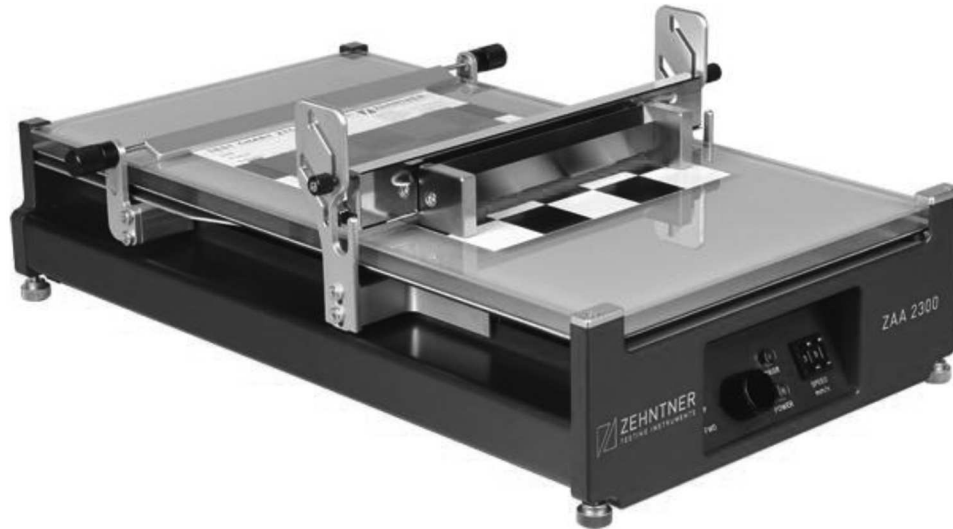
FIG. 3 Blade Film Applicator, Motor-Driven, Practice C
