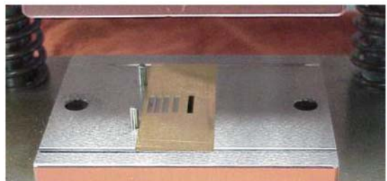
FIG. 4 Narrow Width Specimen – Produced by Stamping
