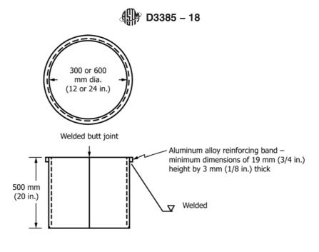
Materials: 3 mm (1/8 in.) aluminum alloy sheet or material of similar strength FIG. 1 Infiltrometer Construction
