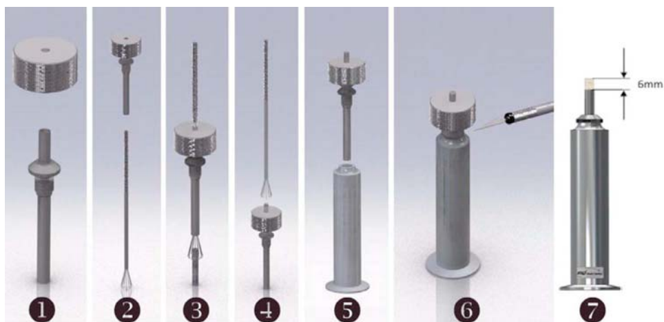
FIG. 5 Wick Positioning Steps
