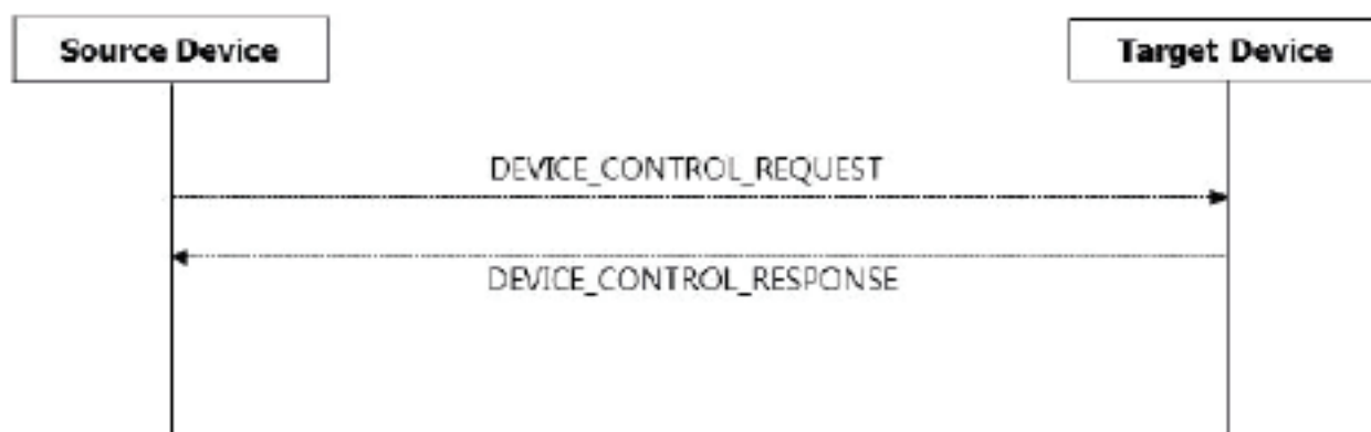
Figure 5 — Device Control Operation
