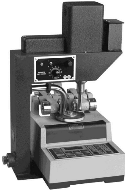
Figure 2 — Example of a Taber abrader with grit feeder
