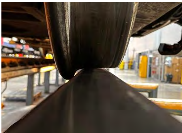
Figure 1 — Demonstration of the size of the contact patch between the wheel and rail
