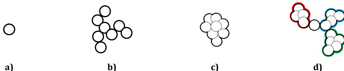
Figure 3 — Various species in a simplified 2D diagram: a) isolated, individual particle, b) agglomerate, c) aggregate, d) agglomerate of three aggregates shown with different colours
